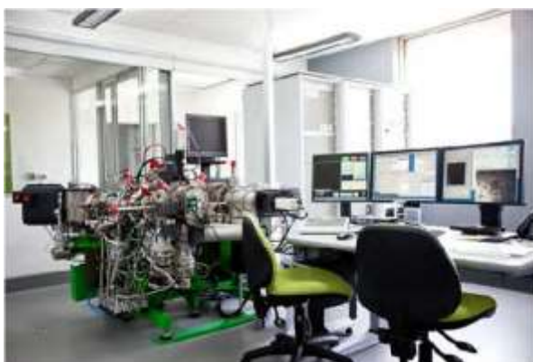
Figure 18: Left: A Secondary Ion Mass Spectrometer (SIMS) used for surface and thin layer chemical analysis. (b) A scanning electron microscope for microscopy and microanalyses. Both tools to be used in the materials characterization laboratory in the hub
