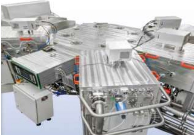
Figure 14: Left: A PECVD for deposition of amorphous silicon or of \text{SiO}_x or \text{SiN} or \text{SiC} or other layers for passivation. Right: Tray used for a Physical Vapor Deposition machine in a solar cell pilot line.
